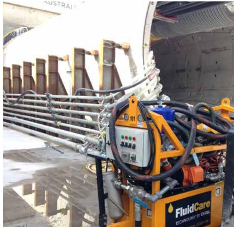
**The process of cleaning the oil, rather than replacing it, had many advantages for Sydney Metro Rail; along with proactively implementing measures to avoid repeat issues.**
